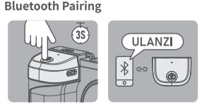
1. Press and hold the shooting button for 3s to turn on the remote control, and the green indicator light flashes. Press and hold for 3s to power off.
