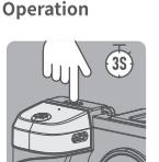
1. Long press the power button for 3s to turn on, the default brightness is 30%. Short press the power button to adjust the brightness, which contains 30%/70%/100% brightness. Long press for 3s to shut down.
