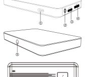
① Type-C charging port ②Switch ③ Color temperature switch ④ Brightness adjustment knob © 1/4 expansion screw hole © LED Indicator
